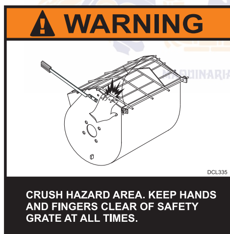
Figure 42. Safety Grate (Crush Hazard)
