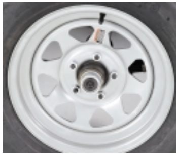
Wheel Bearing Grease Fittings Offers convenient wheel bearing lubrication thru zerk fittings.
