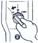
3. Turn the fuel valve to the "OFF" position.
