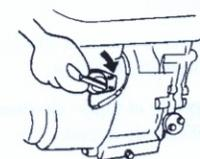
5. Pull the starter grip lightly until resistance is felt, then pull briskly.
