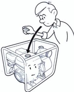
2. If the fuel level is low. Fill to the shoulder of the fuel filter.
