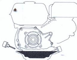
3. Tighten the oil drain plug and fill the oil to the edge of the oil filler neck.
