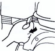
3. Turn the choke lever to the close position.
