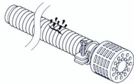
Is the hose band installed securely?
